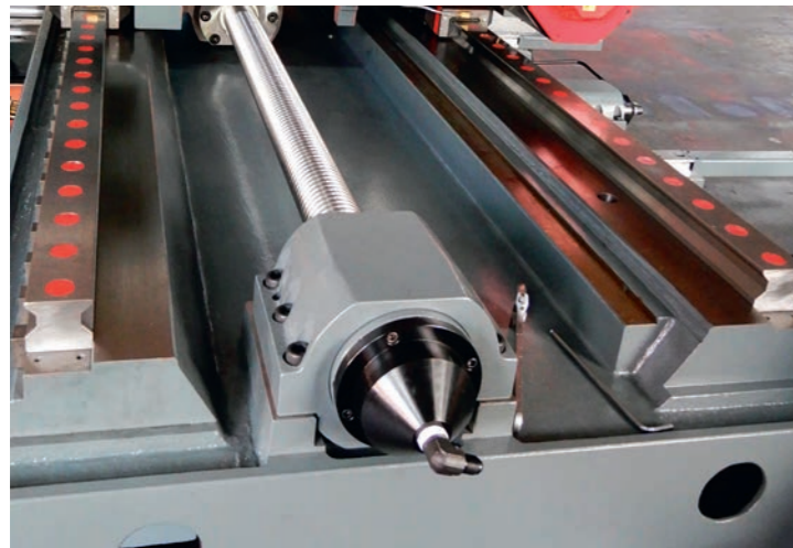
X axis linear guideway Optional : Ball screw with hollow cooling system
